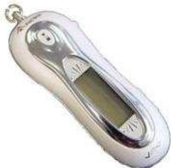
Figure 6.2: This picture shows the Frontel MP301 MP3 player, measuring 8.5 \times 3.2 \times 1.8 cm and weighing 37 grams. (from: http://frontelinc.com.tw/product/mp200.htm )
