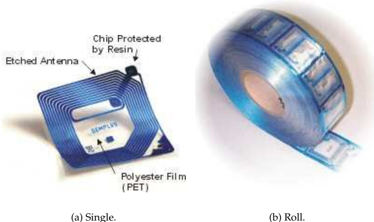
Figure 6.1: Example of a RF tag, available on peel-and-stick rolls with each tag measuring 4 \times 4 \times 0.1 cm.
